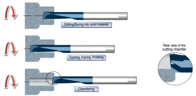
The tool is equipped with an additional cutting edge, which is located across the main front edge. This allows production of an additional 45° chamfer on the work piece without the need to stop the spindle or processing operation.
